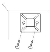
11. Attach intermediate tubing to cable supports with the cable ties between soap pumps
