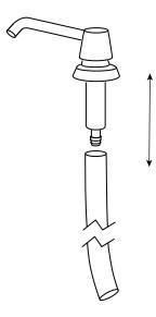
4. Insert soap pump assemblies with vertical tubes into Shanks.
