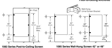
These mounting points require backing. For suggested backing methods, Bobrick Advisory Bulletins TB-32 for ceiling-hung installations and TB-46 for flooranchored are available upon request
