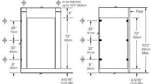
These mounting points require backing. For suggested backing methods, Bobrick Advisory Bulletins TB-32 for ceiling-hung installations and TB-46 for floor-anchored are available upon request.
