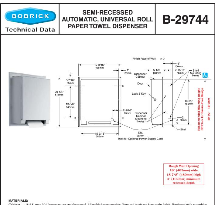
**Cabinet** — 18-8 S, type-304, heavy-gauge stainless steel. All-welded construction. Exposed surfaces have satin finish. Equipped with a tumbler lock keyed like other Bobrick washroom accessories.
