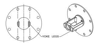
Next carefully slide yoke assembly into body and around pilot seat.
