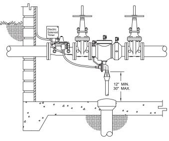
Model 375MS with ZW206 Solenoid Control Valve and EST
