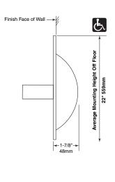
Rough Wall Opening 5-1/4" (133mm) Wide 5-1/4" (133mm) High 2-1/2" (63mm) minimum recessed depth
