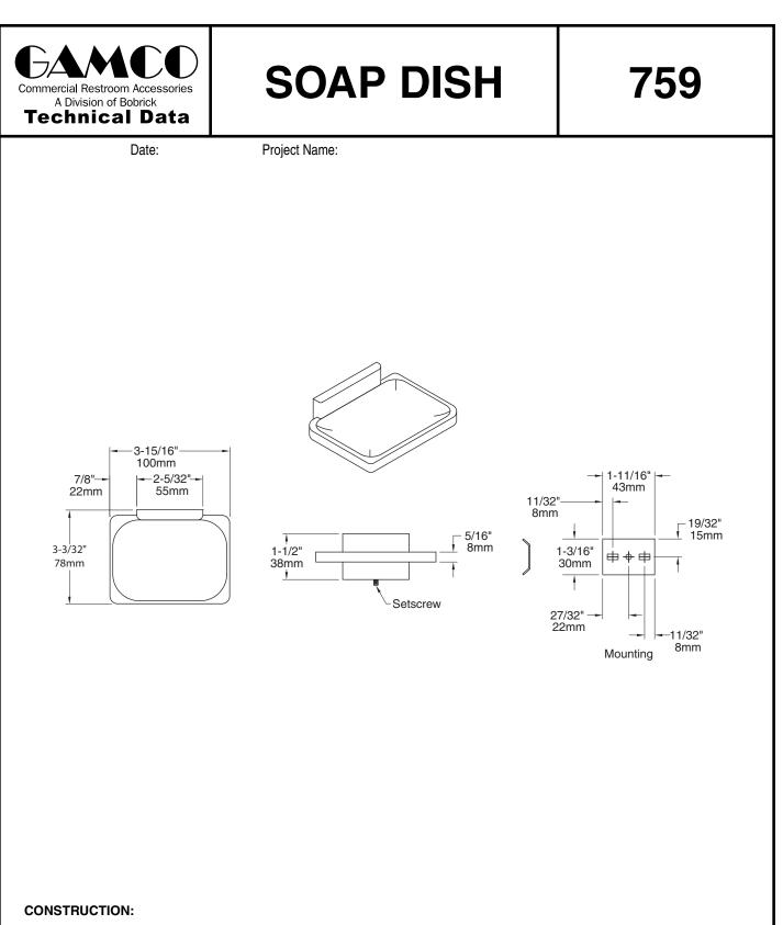
Soap dish is die-cast from highest quality virgin zinc alloy (Zamak) to meet ASTM standard B-86. Castings are highly polished and plated with chrome. Wall plate is 18-gauge (1.2mm) zinc-plated steel.
