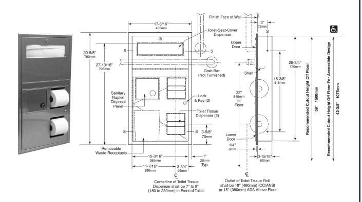
Rough Wall Opening 16" (405mm) wide 29-1/4" (745mm) high 4" (102mm) minimum recessed depth
