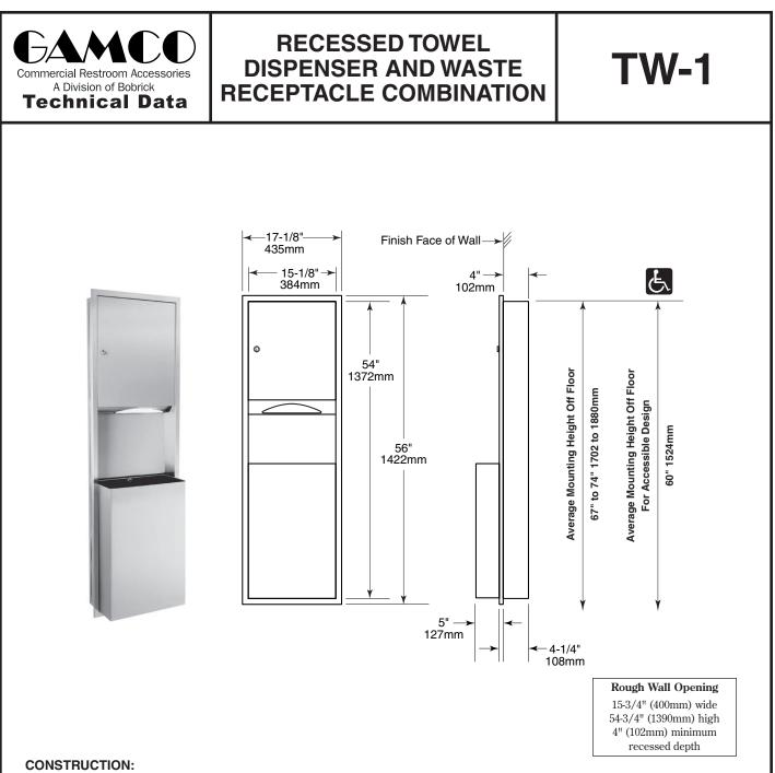
Fabricated type 304 heavy-gauge stainless steel. All welded construction with exposed surfaces having a #4 satin-finish. One piece seamless 22-gauge (0.8mm) flange provided with 1/4" (102mm) return for rigidity. EXTRA HEAVY 18-gauge (1.2mm) door, warp free, hung on continuous stainless steel piano-hinge, and fitted with tumbler lock. Waste receptacle is 22-gauge (0.8mm) and secured to cabinet with tumbler lock and is removable for servicing; top and bottom edges hemmed for safe handling.
