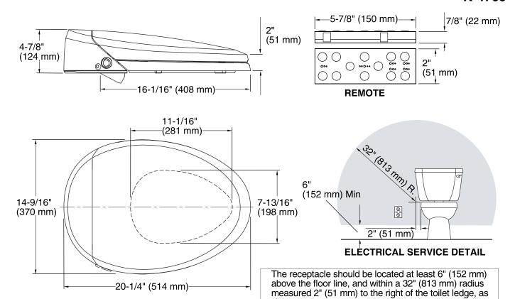
One dedicated circuit required, protected with Class A Ground-Fault Circuit-Interrupter (GFCI) or Residual Current Device (RCD).
